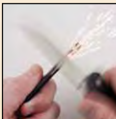
Run the back of the blade along the flint rod for fire starting.
